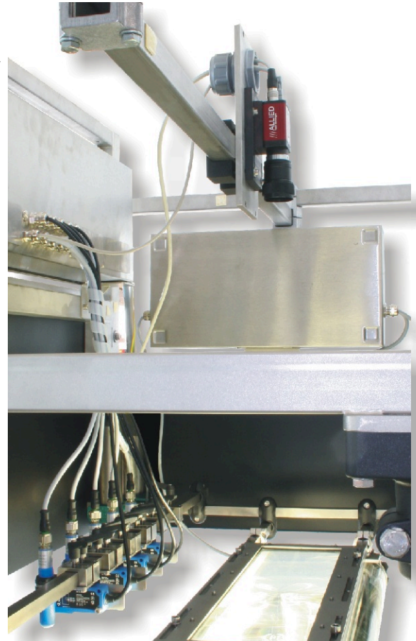
CCD-Firewire-Camera and sensors in one sensor bridge
